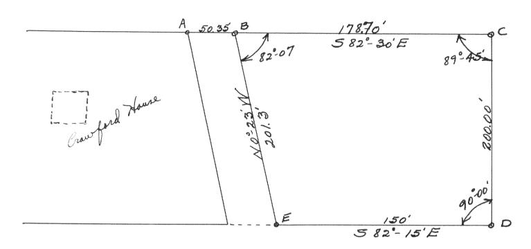
Survey of a small piece for R.M. Crowford Joeation - Gerois the road from R.M. Crowford's residence on Kelavan Jake in the ME & see 27, T27, R16E Monuments - Found iron pipe at A Froedure - measured and set iron pipes as shown on sketch, the property him lasted directly east of R. M. Crawford's lake Shore property.
