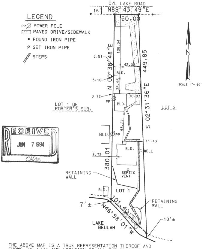
THE ABOVE MAP IS A TRUE REPRESENTATION THEREOF AND SHOWS THE SIZE AND LOCATION OF ALL THE PROPERTY, EXTERIOR BOUNDARIES, THE LOCATION OF ALL VISIBLE BOUNDARY FENCES, APPARENT EASEMENTS, ROADWAYS AND VISIBLE ENCROACHMENTS, IF ANY.
