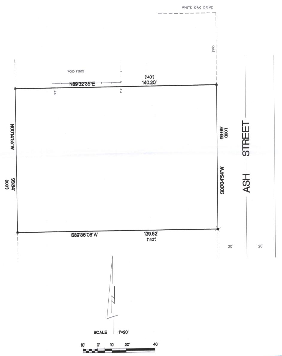
BEARINGS ARE REFERENCED TO THE EAST LINE OF THE NORTHEAST 1/4 OF SECTION 10-4-18 AND IS ASSUMED TO BEAR NOO"15'42"W, (NAD83).
