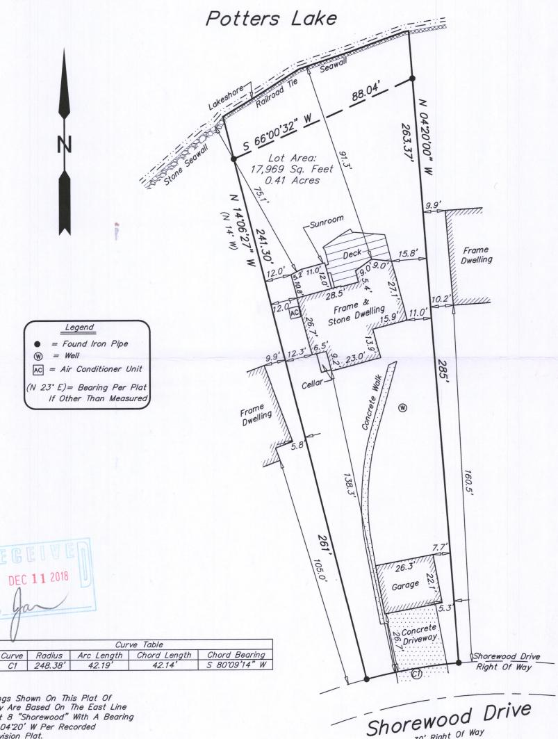
Bearings Shown On This Plat Of Survey Are Based On The East Line Of Lot 8 "Shorewood" With A Bearing Of N 04°20' W Per Recorded Subdivision Plat.
