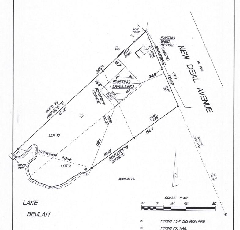
BEARINGS ARE REFERENCED TO THE NORTH LINE OF THE NORTHWEST 1/4 OF SECTION 18-4-18 AND IS ASSUMED TO BEAR N89'02'08"E, NAD 1927.
