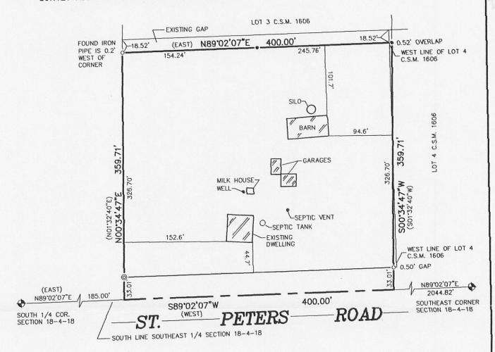
BEARINGS HEREON RELATE TO THE SOUTH LINE OF THE SOUTHEAST 1/4 OF SECTION 18-4-18. ASSUMED BEARING IS NORTH 89'02'07" EAST.
