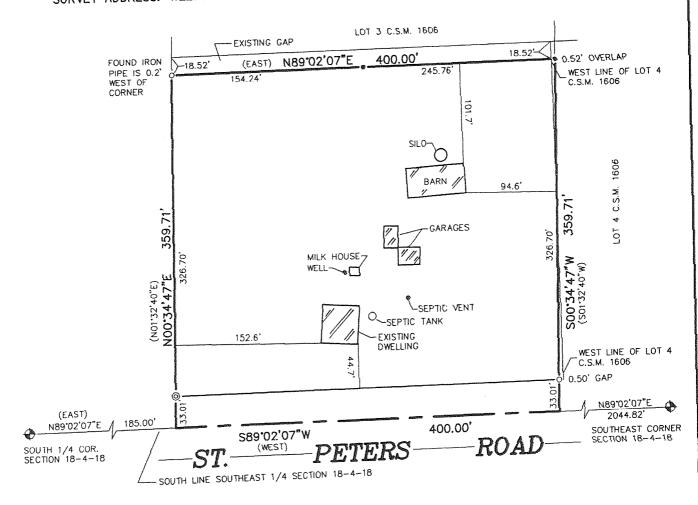
BEARINGS HEREON RELATE TO THE SOUTH LINE OF THE SOUTHEAST 1/4 OF SECTION 18-4-18. ASSUMED BEARING IS NORTH 89'02'07" EAST.
