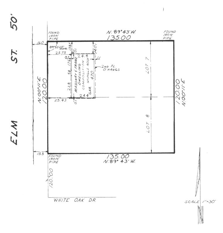
1 Certify that I have surveyed the above described property (Property), and the above map is a true representation thereof and shows the size and location of the Property, its exterior boundaries, the location and dimensions of all visible structures thereon, boundary fences, apparent easements and roadways and visible encroachments, if any.
