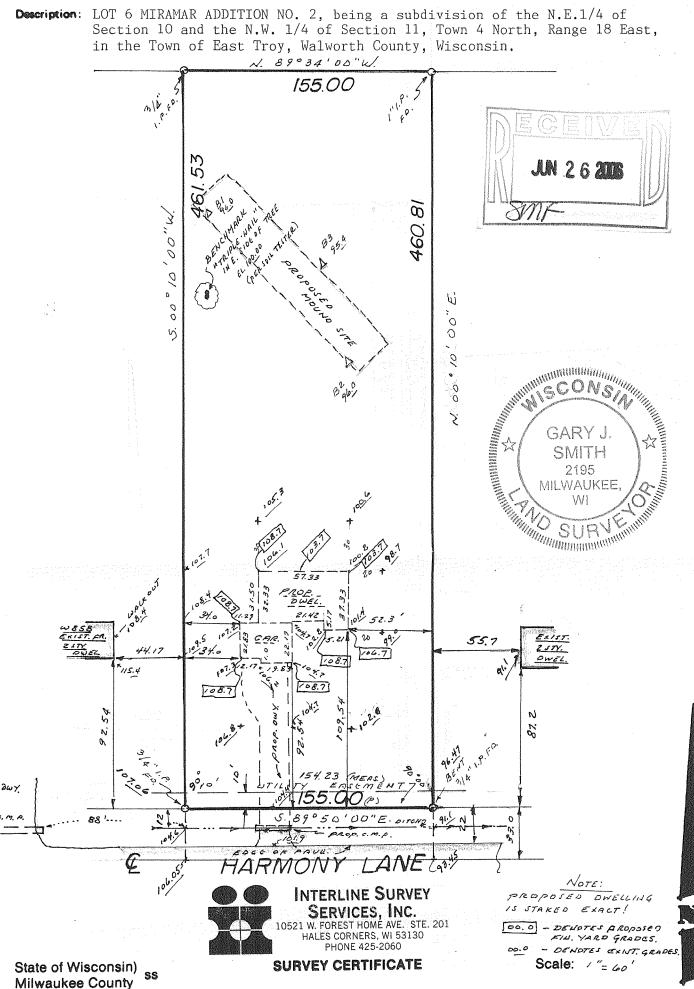
We, Interline Survey Services, Inc., certify that we have surveyed the above described property and the above map is a true representation thereof, and shows the size and location of the property, its exterior boundaries, the location and dimensions of all visible structures thereon, fences, apparent easements and roadways and visible encroachments, if any.
