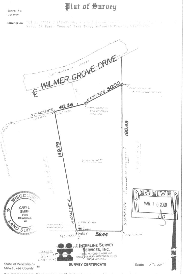
We, Interline Survey Services, Inc., certify that we have surveyed the above described property and the above map is a true representation thereof, and shows the size and location of the property, its exterior boundaries, the location and dimensions of all visible structures thereon, fences, apparent easements and roadways and visible encroachments, if any.
