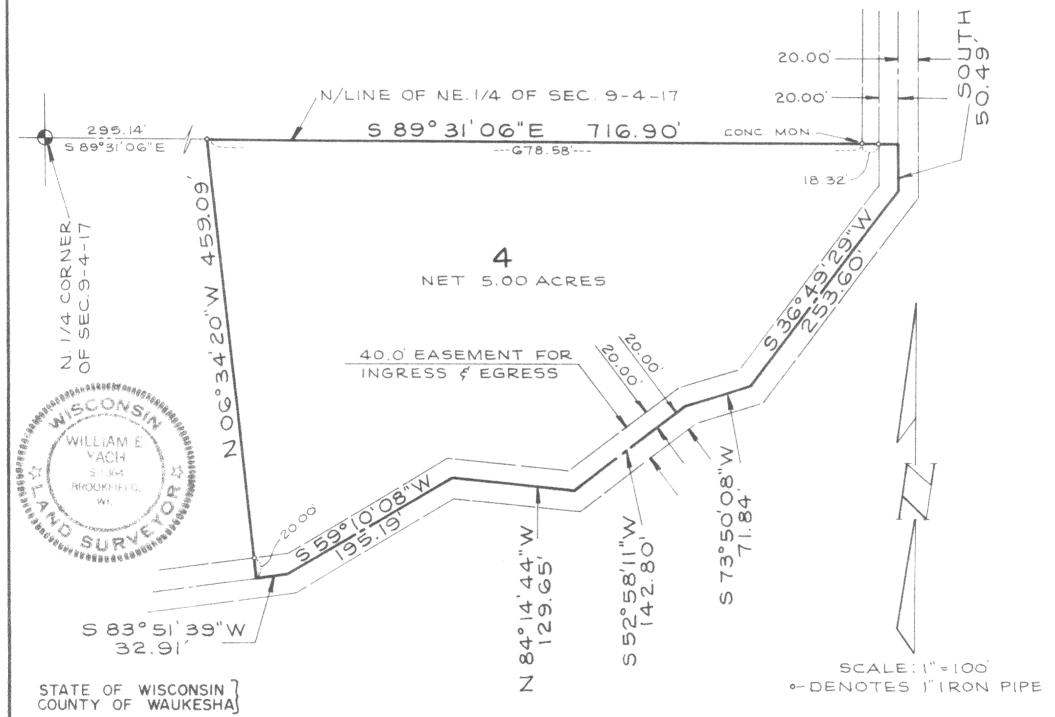
I hereby certify that I have surveyed the above described property and the above map is a true representation thereof and shows the size and location of the property, its exterior boundaries, the location of all visible structures and dimensions of all principle buildings thereon, boundary fences, apparent easements, roadways and visible encroachments, if any.
