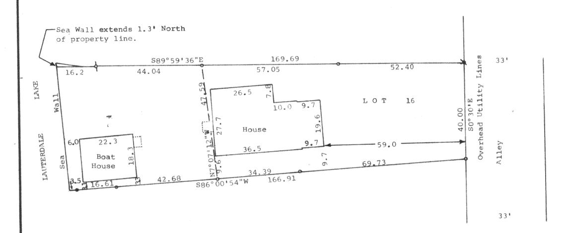
Scale - 1" = 20o = 1" Dia. Iron Pipe Found ♦ = ½" Dia. Iron Rod Found i = 3/4" Dia. Iron Pipe Found Bent and reset • = 3/4"x24" Iron Pipe Set
