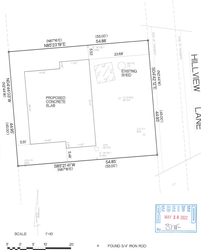
BEARINGS ARE REFERENCED TO THE WEST LINE OF THE NORTHWEST 1/4 OF SECTION 25-4-16 AND IS ASSUMED TO BEAR N01°10'48"E, (NAD83).
