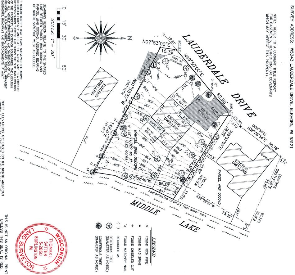
NOTE: ELEVATIONS ARE BASED ON THE NORTH AMERICAN VERTICAL DATUM OF 1988. THE 100 YEAR FLOOD LINE ELEVATION FOR MIDDLE LAKE BASED ON SAID DATUM IS 88.6' PER SUMMARY OF STILLWAITER ELEVATIONS PUBLISHED BY FEMA. THE MEAN ELEVATION FOR THE APPROXIMATED ORDINARY HIGH WAITER MARK USED BY THIS OFFICE WAS 885.3'. ONLY THE LINE FOR THE APPROXIMATED ORDINARY HIGH WAITER MARK IS SHOWN HEREON, SINCE THERE IS A RELATIVELY SUBSTANTIAL LAKE BANK AND THE TWO LINES LIE CLOSELY TOGETHER.
