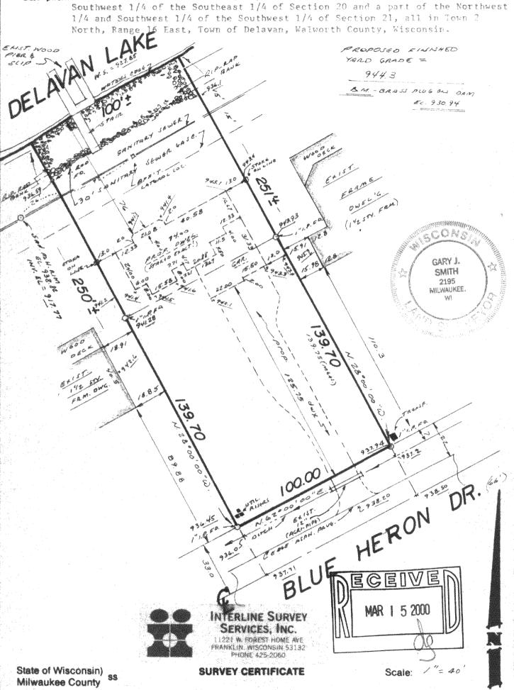
We, Interline Survey Services, Inc., certify that we have surveyed the above described property and the above map is a true representation thereof, and shows the size and location of the property, its exterior boundaries, the location and dimensions of all visible structures thereon, fences, apparent easements and roadways and visible encroachments, if any.
