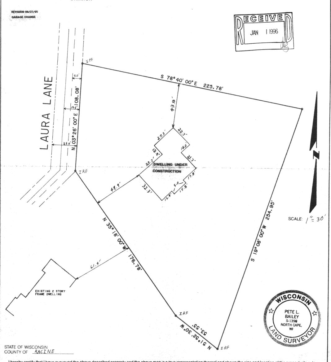
I hereby certify that I have surveyed the above described property and the above map is a true representation thereof and shows the size and location of the property, its exterior boundaries, the location of all visible structures and dimensions of all principle buildings thereon, boundary fences, apparent easements, roadways and visible encroachments, if any.
