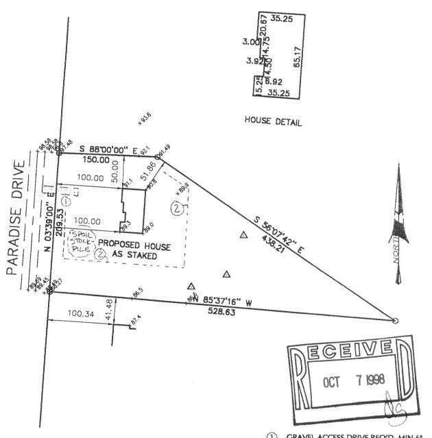
① GRAVEL ACCESS DRIVE REQ'D. MIN 6" DEPTH, 2" TO 3" AGG. 10' WIDE X 50 L.F.
