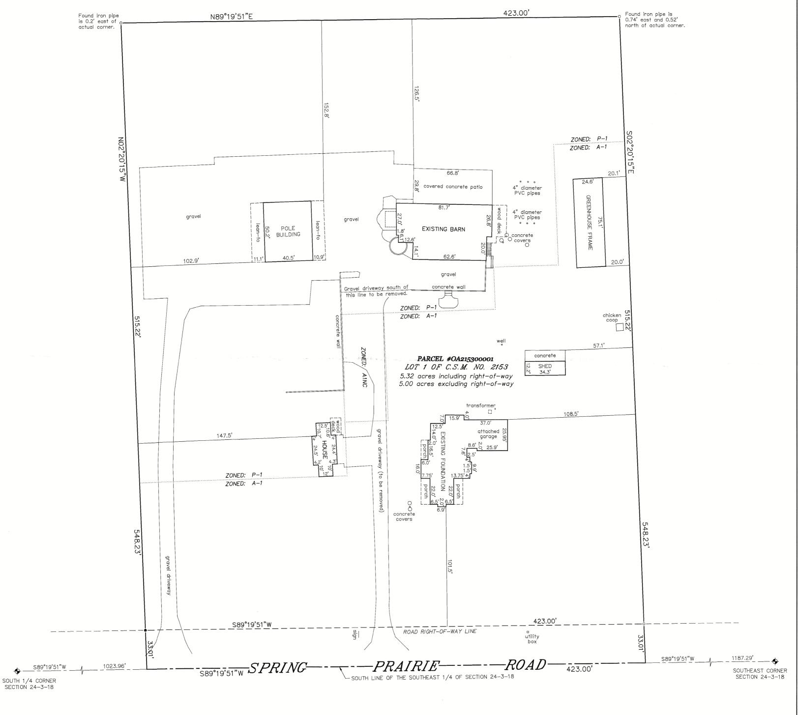
BEARINGS HEREON RELATE TO GRID NORTH OF THE WISCONSIN STATE PLANE COORDINATE SYSTEM, SOUTH ZONE (NAD-1927). ASSUMED BEARING OF SOUTH 89°19'51" WEST ON THE SOUTH LINE OF THE SOUTHEAST 1/4 OF SECTION 24-3-18 AS PLATTED.
