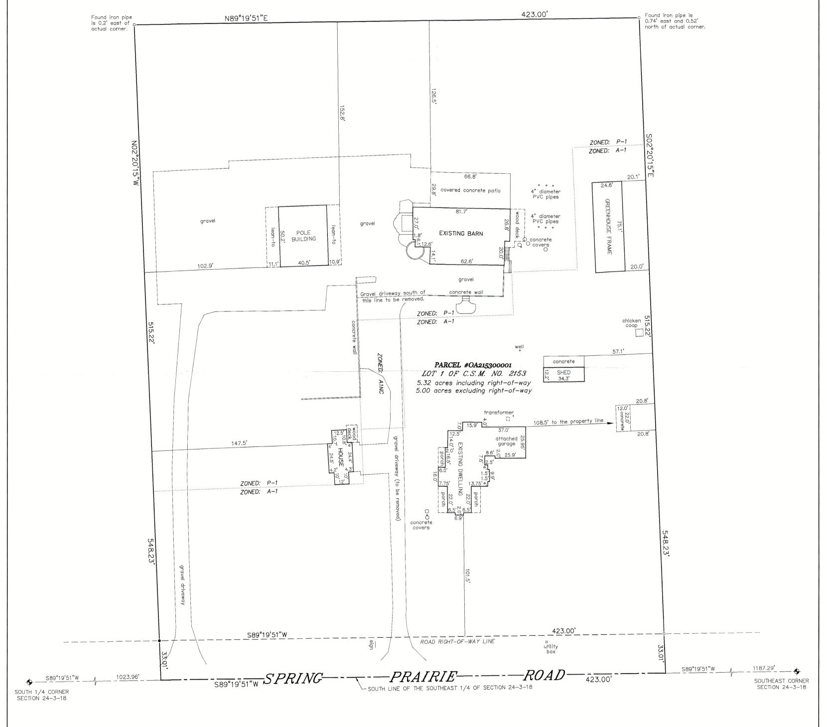
BEARINGS HEREON RELATE TO GRID NORTH OF THE WISCONSIN STATE PLANE COORDINATE SYSTEM, SOUTH ZONE (NAD-1927). ASSUMED BEARING OF SOUTH 89°19'51" WEST ON THE SOUTH LINE OF THE SOUTHEAST 1/4 OF SECTION 24-3-18 AS PLATTED.
