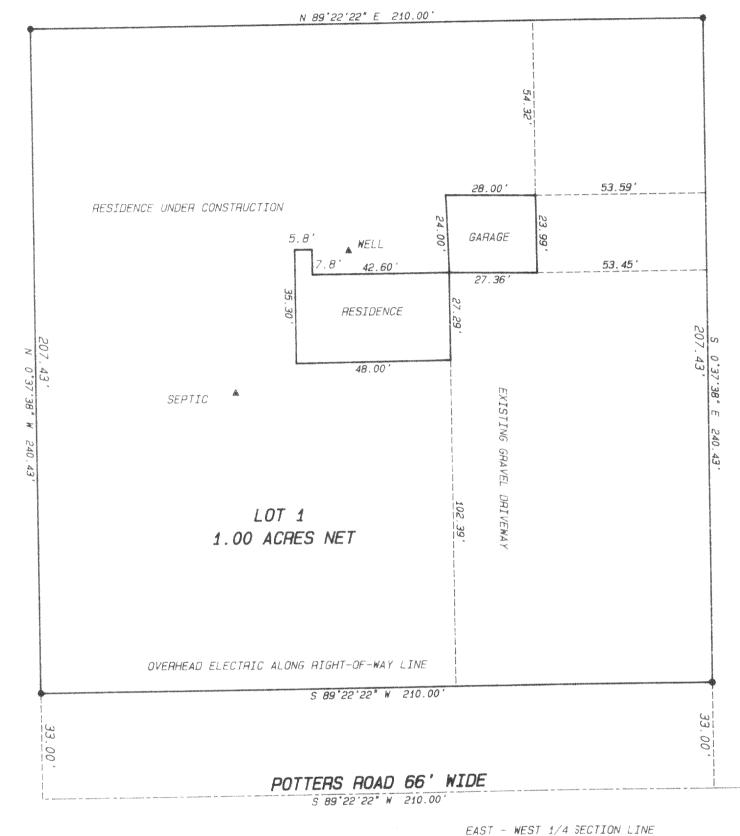
NOTE: EXISTING RESIDENCE AS PREVIOUSLY SHOWN ON CSM HAS BEEN REMOVED AND REPLACED BY A NEW FOUNDATION AS SHOWN.
