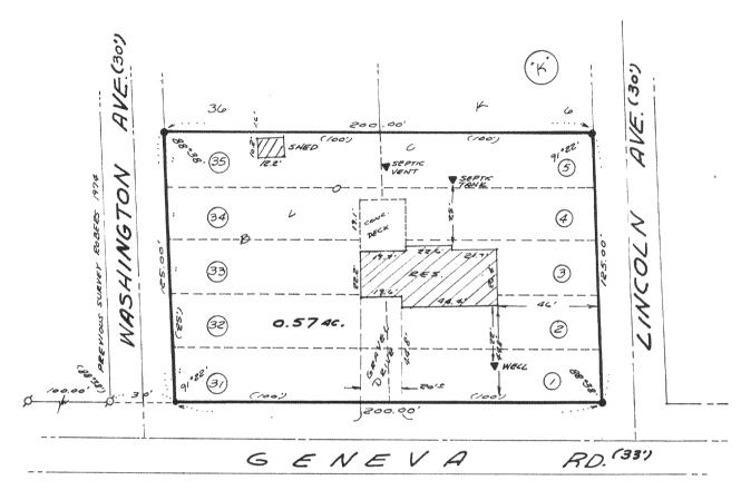
note: found bent irion pipe at NW Cor. Lot 35 and reset iron rod. This agreed with previous survey in Block "L".
