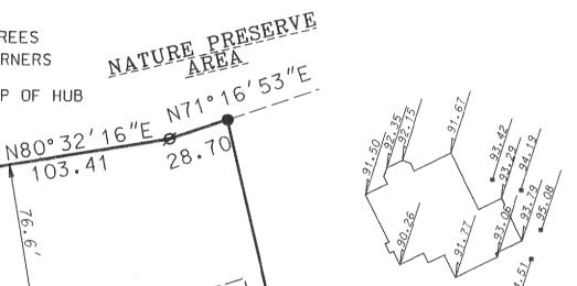
ELEVATION AT CORNERS AND AT TOP OF HUB 10' FROM CORNER BASED ON ASSUMED ELEVATION OF 100.00 AT SOUTHWEST CORNER OF LOT.
