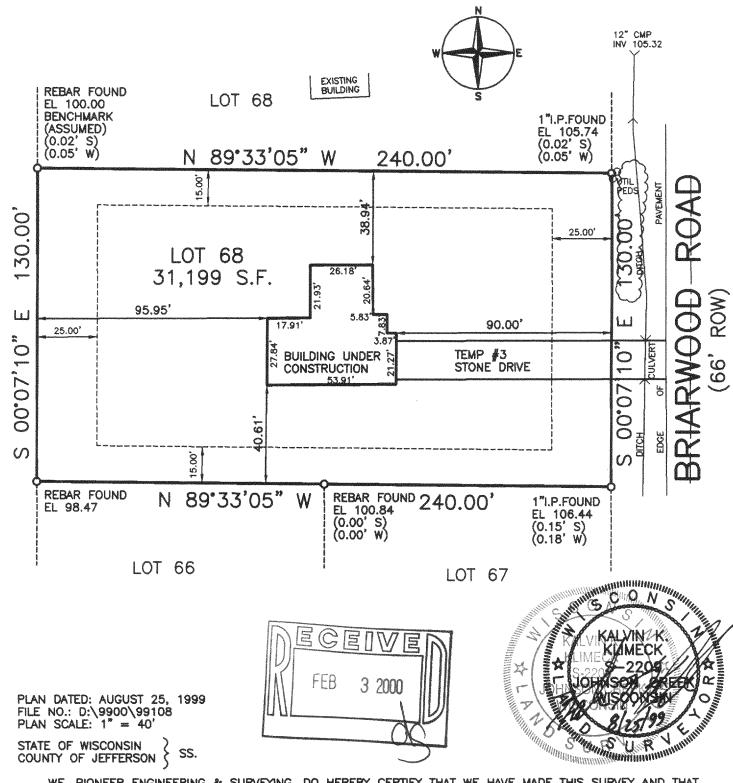
WE, PIONEER ENGINEERING & SURVEYING, DO HEREBY CERTIFY THAT WE HAVE MADE THIS SURVEY AND THAT THE INFORMATION AS SHOWN ON THE ABOVE PLAT OF SURVEY IS TRUE AND CORRECT REPRESENTATION THEREOF.
