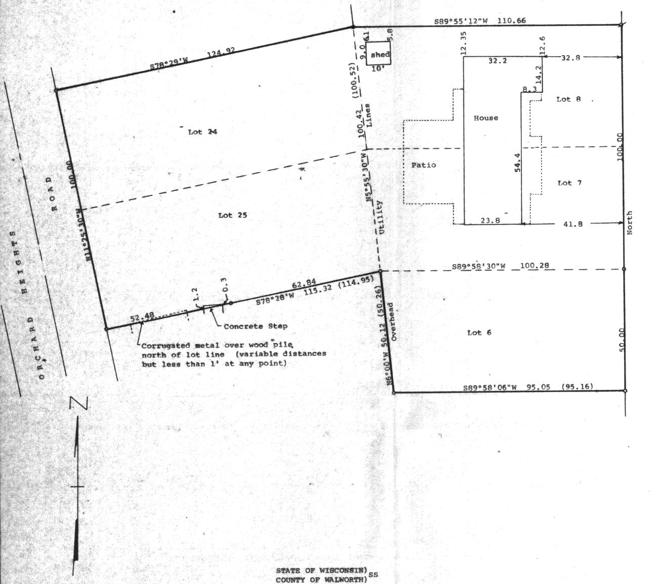
Scale - 1" = 20° o = 5/8" Iron Rod Found = 5/8" Iron Rod Found bent and reset
