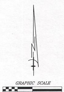
BEARINGS HEREON RELATE TO GRID NORTH OF THE WISCONSIN STATE PLANE COORDINATE SYSTEM (SOUTH ZONE).
