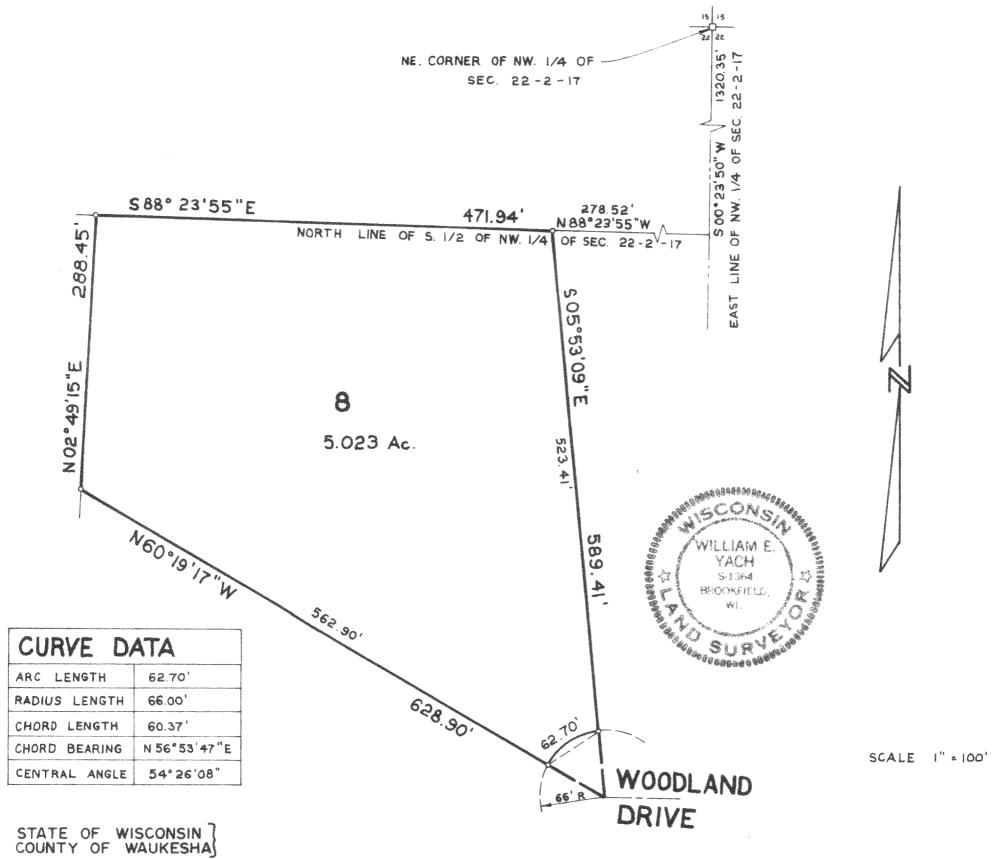
I hereby certify that I have surveyed the above described property and the above map is a true representation thereof and shows the size and location of the property, its exterior boundaries, the location of all visible structures and dimensions of all principle buildings thereon, boundary fences, apparent easements, roadways and visible encroachments, if any
