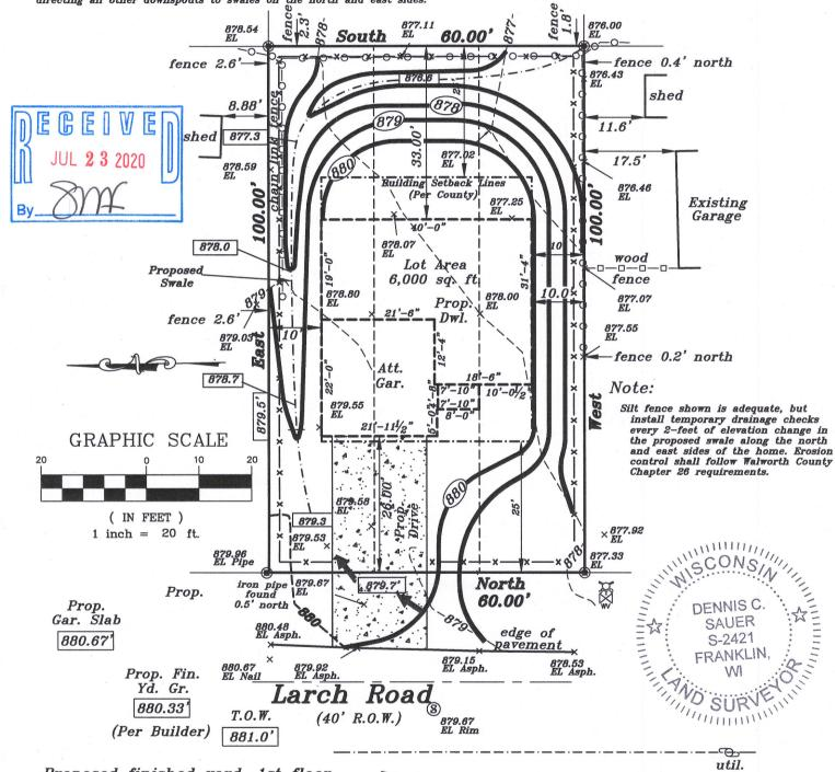
Proposed finished yard, 1st floor or top of foundation grade shown on this drawing is a suggested grade and should be verified by the owner, builder or municipality
