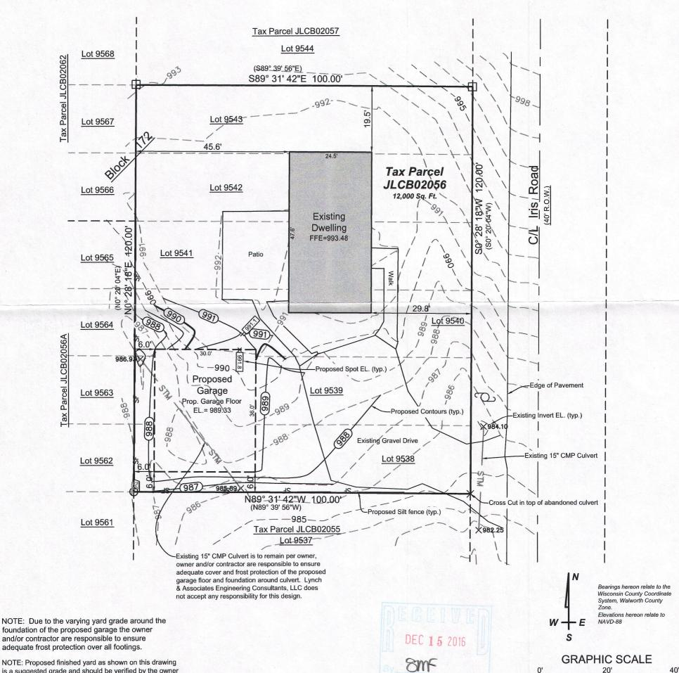
NOTE: Proposed finished yard as shown on this drawing is a suggested grade and should be verified by the owner and/or the builder and approved by the building inspector. Erosion control measures are suggested and must be verified/adjusted by the builder and/or building inspector
