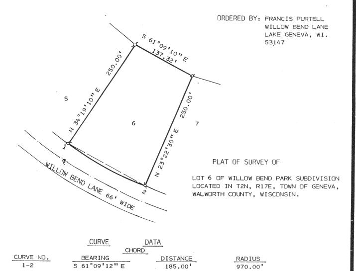
NOTE: BEARINS ARE TIED TO THE WISCONSIN COORDINATE SYSTEM AS SHOWN ON THE RECORDED PLAT.
