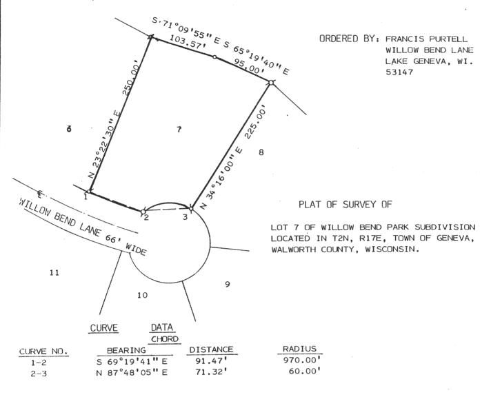
NOTE: BEARINGS ARE TIED TO THE WISCONSIN COORDINATE SYSTEM AS SHOWN ON THE RECORDED PLAT.
