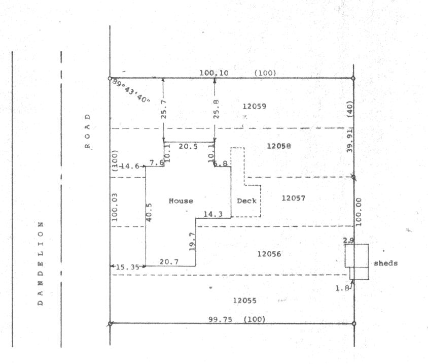
Scale - 1" = 20"O = 1" Iron Pipe Found X = 1" Iron Pipe Found  $\emptyset = \frac{1}{2}$ " Iron Pipe Found 1' below ground (0.00) = recorded distance
