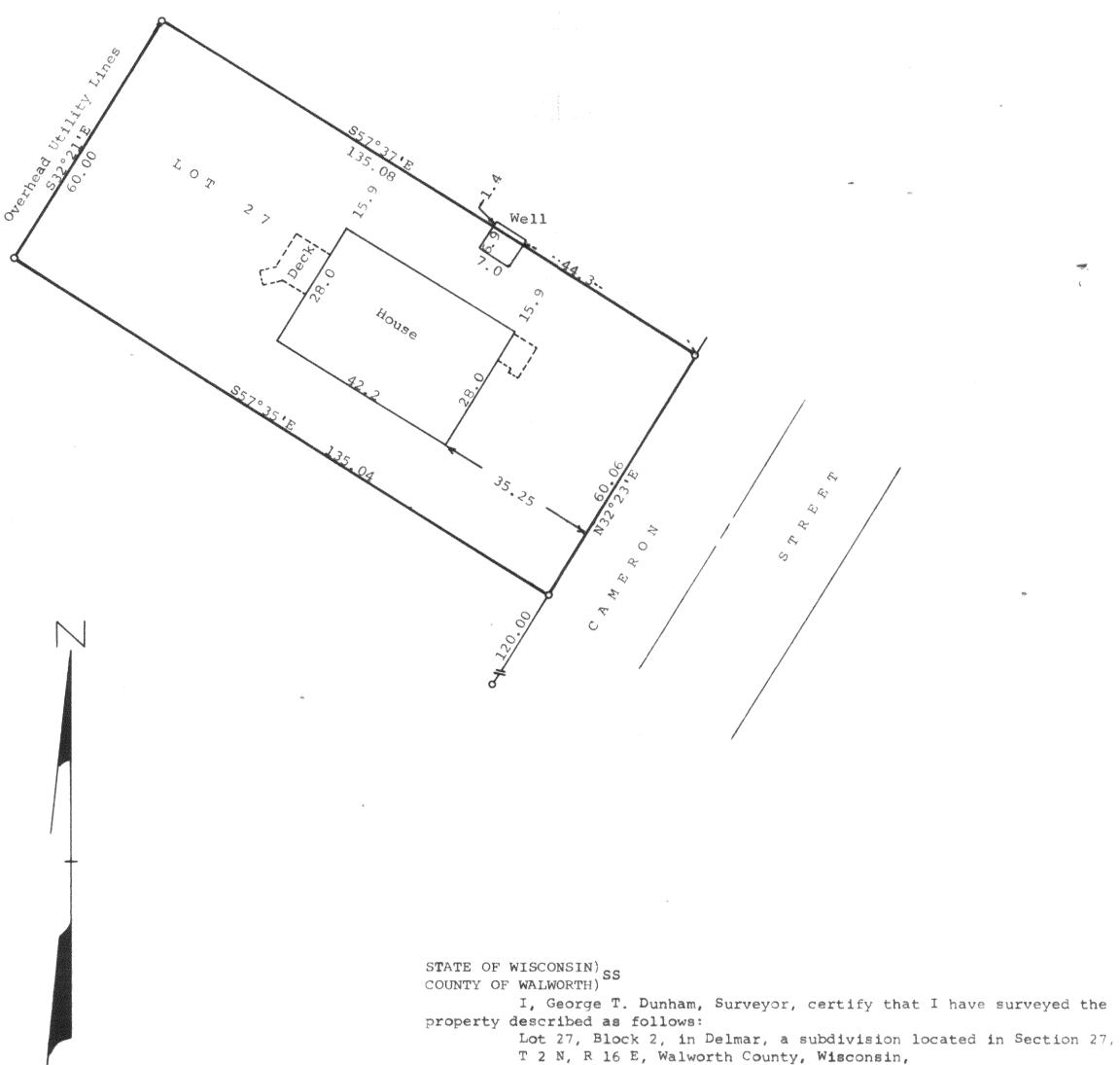
Scale - 1" = 20' •= 1" Iron Pipe Found Bearings referenced to the recorded bearing of N32°23'E along the northwesterly line of Cameron Street Survey ordered by: Realty World Carmin Realtors 811 East Geneva Street Delavan, WI 53115
