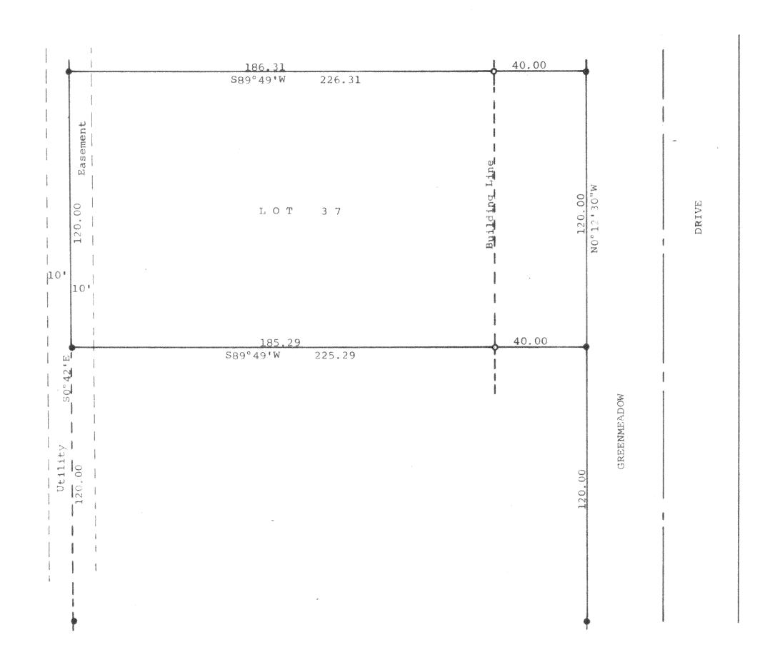
Scale - 1" = 30"•= 11/16" Diameter Iron Rod Found. O = ½" X 24" Iron Pipe Set Bearings used are those of record Survey ordered by: Century 21, Skandia Realty 312 South 7th Street Delavan, WI.593135
