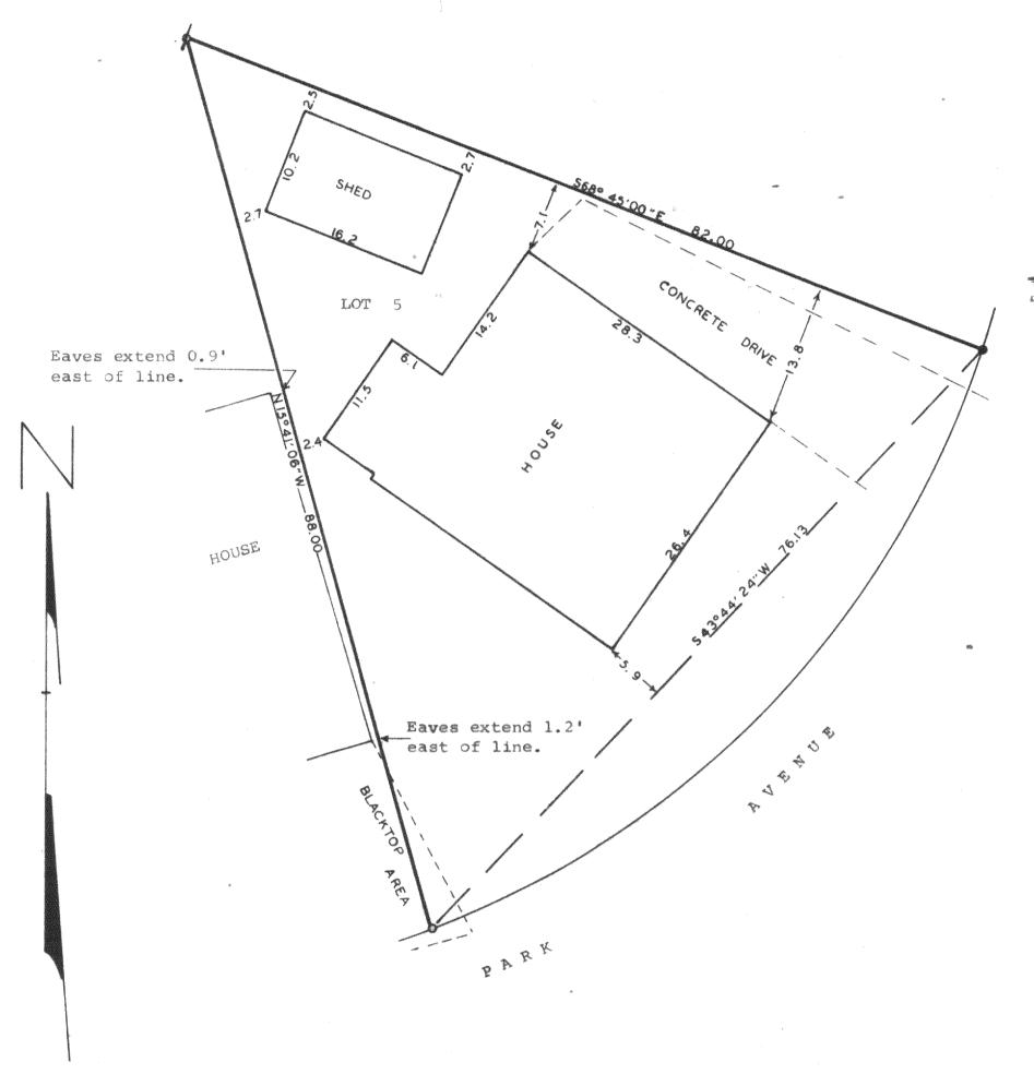
Scale ~ 1" = 10' ≠ 3/4" Dia. Iron Pipe Found • = 14" Dia. Iron Pipe Found • = Iron Pipe Set 3/4"x24"
