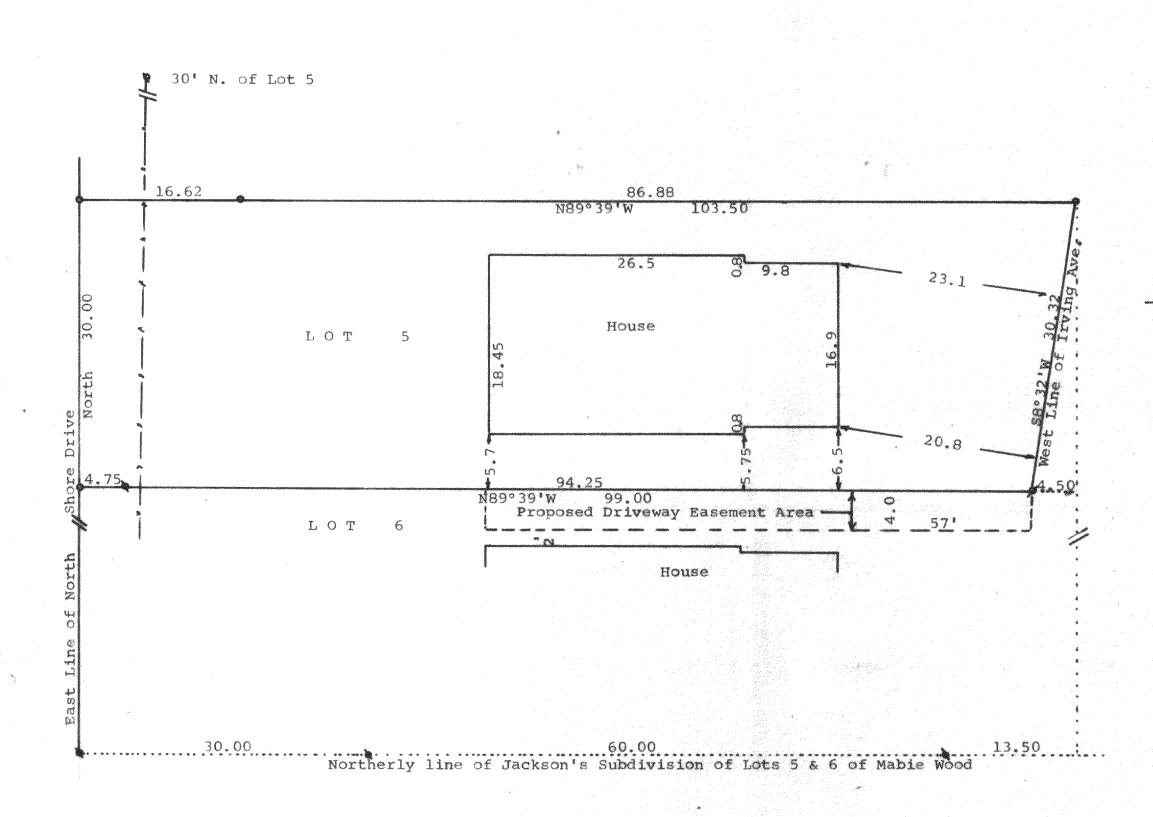
Scale - 1" = 10"= 3/4" Iron Pipe Found • = 3/4" X 24" Iron Pipe Set ---- Fence Line Bearings referenced to the assumed bearing of North along the east line of North Shore Drive Survey ordered by: Turner Realty 1815 North Shore Drive Delavan, WIsconsin 53115
