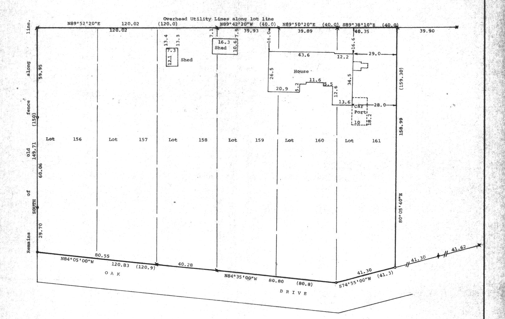
Note: Bearings are referenced to the West line of Lot 156, recorded Bearing is South.
