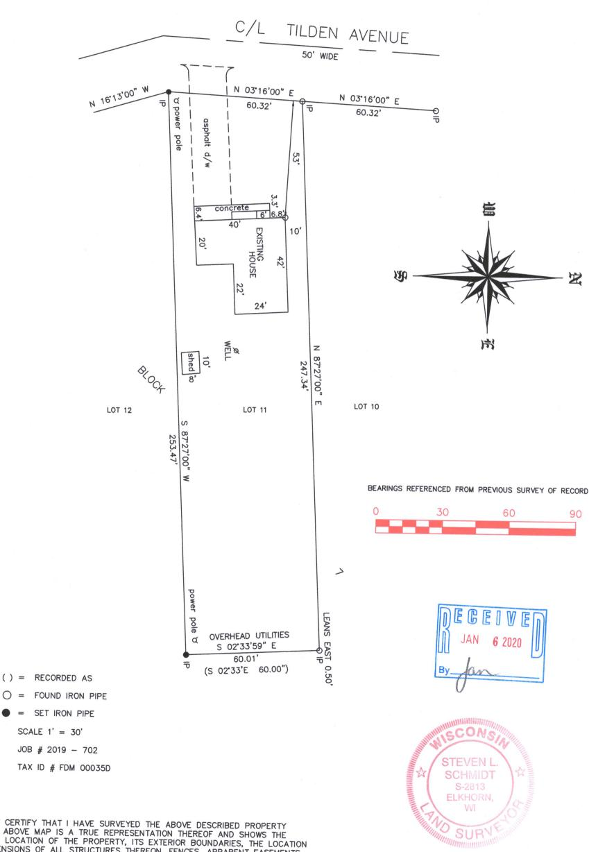
I HEREBY CERTIFY THAT I HAVE SURVEYED THE ABOVE DESCRIBED PROPERTY AND THE ABOVE MAP IS A TRUE REPRESENTATION THEREOF AND SHOWS THE SIZE AND LOCATION OF THE PROPERTY, ITS EXTERIOR BOUNDARIES, THE LOCATION AND DIMENSIONS OF ALL STRUCTURES THEREON, FENCES, APPARENT EASEMENTS AND ROADWAYS AND VISIBLE ENCROACHMENTS IF ANY.
