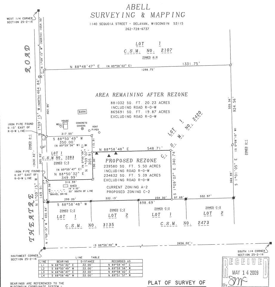
WISCONSIN COORDINATE SYSTEM -SOUTH ZONE, DATUM NAD 1927. THE BEARING OF THE SOUTH LINE OF THE SOUTHWEST 1/4 IS S 88°58'48" W
