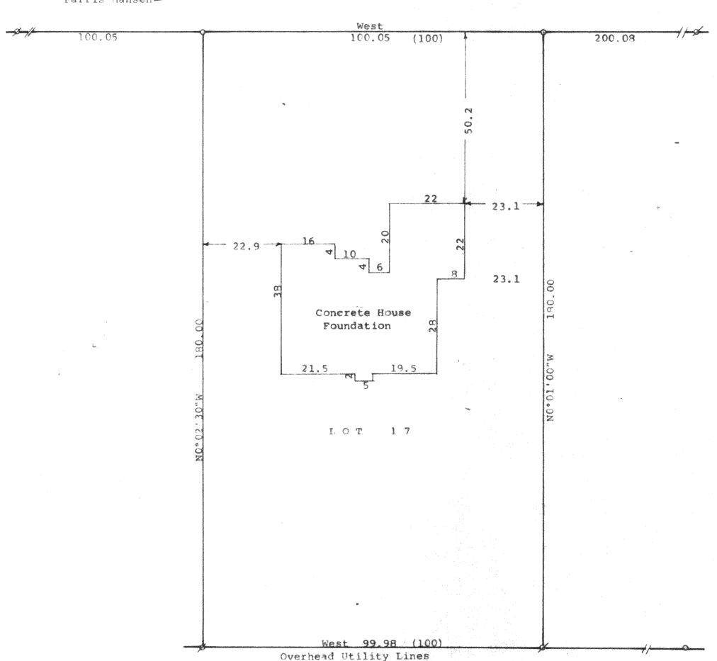
Scale - 1" = 20" $\emptyset$ = 1" Iron Pipe Found o= 1" Iron Pipe Set Bearings are referenced to the south line of Vælencia Street with the recorded bearing of East-West Survey ordered by: Gordon Nelson For Warren Bentley c/o Professional Realty 706 East Geneva Street Delavan, WI 53115 (.00) = recorded distance
