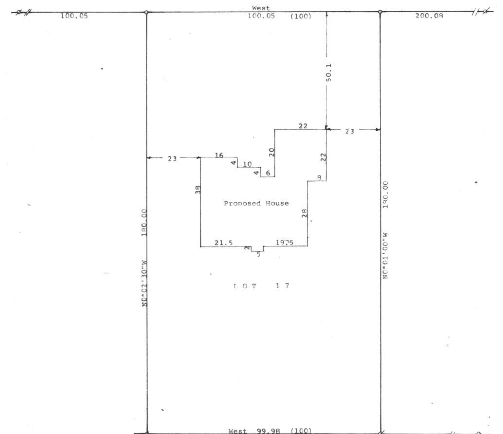
Scale - 1" = 20" $\emptyset = 1$ " Iron Pipe Found o= 1" Iron Pipe Set Bearings are referenced to the south line of Valencia Street with the recorded bearing of East-West Survey ordered by: Gordon Nelson For Warren Bentley c/o Professional Realty 706 East Geneva Street Delavan, WI 53115 (.00) = recorded distance
