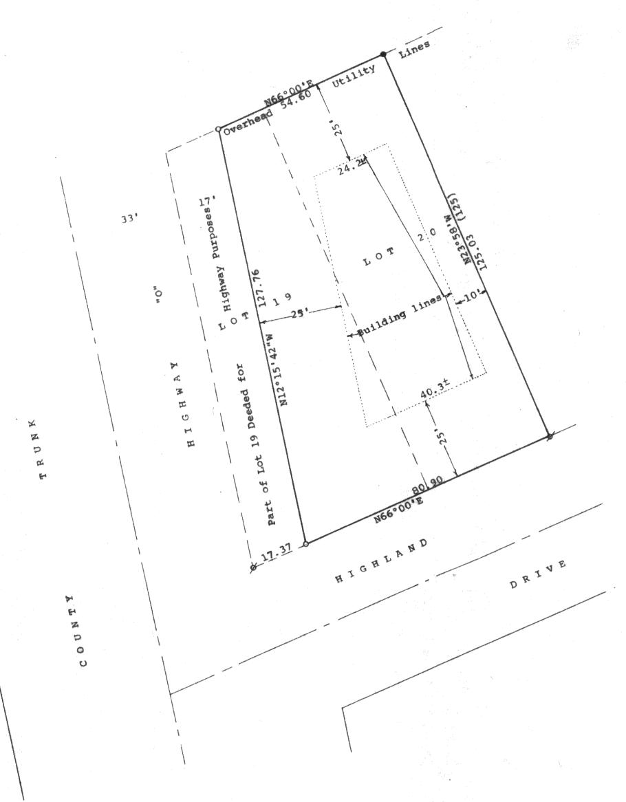
Scale -1" = 20"•= 1½" Iron Pipe Found  $\emptyset = 3/4$ " Iron Pipe Found 0 = 3/4" X 24" Iron Pipe Set Bearings referenced to the assumed bearing of N66°00'E along the northerly line of Highland Drive Survey ordered by: Century 21, Skandia Realty 312 South 7th Street Delavan, WI 53115 (0.00) = recorded distance Updating and recertification ordered by: Mitch Bugno 3527 Hobbs Drive
