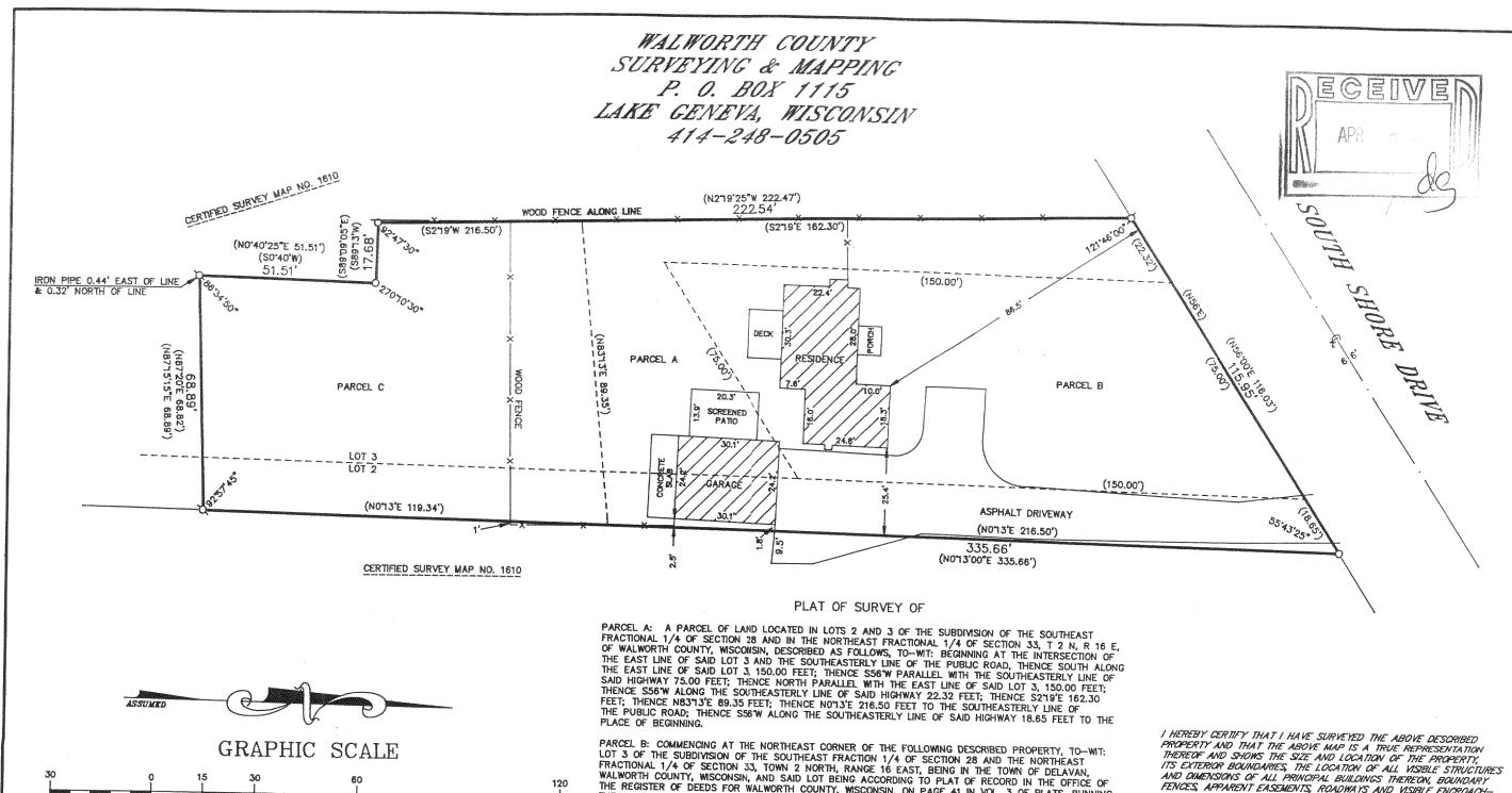
( IN FEET ) 1 inch = 30 ft.Ø-IRON PIPE FOUND Ø-IRON ROD FOUND **■**-CONCRETE MONUMENT FOUND O-IRON PIPE PLACED ()-RECORDED AS
