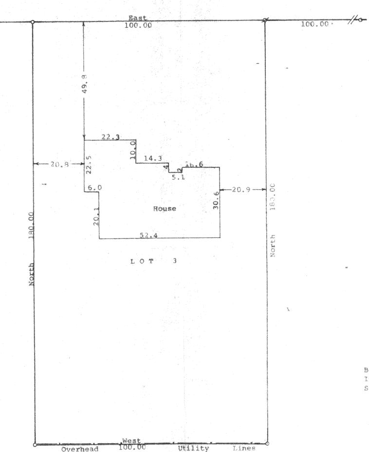
Scale - 1" \* 20' ○ \* 1" Iron Pipe Found Ø = bent 1" Iron Pipe Found. Pulled and reset 1" X 24" Iron Pipe ----- old Fence Line
