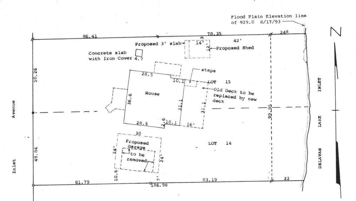
Scale - 1" = 20' Ø= 1" Iron Pipe Found 0 = 3/4" Iron Pipe Found •= 11 Iron Pipe Found Survey ordered by:
