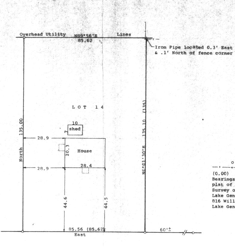
Scale - 1" = 20' O = 1" Iron Pipe Found ------ Fence Line (0.00) = recorded distance Bearings are those given on the recorded plat of Delmar Survey ordered by: Lake Geneva Properties 816 Williams Street Lake Geneva, WI 53147
