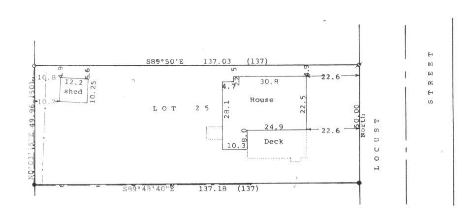
Scale - 1" = 20'0 = 1" Iron Pipe Found Ø = 14" Iron Pipe Found • = 5/8" Iron Rod Found - remains of old wire fence -v-= wire fence - = wood fence (0.00) = recorded distance Bearings referenced to the west line of Locust Street with the assumed bearing of North, Survey ordered by: Tom Glista 4121 Locust Delavan, WI 53115
