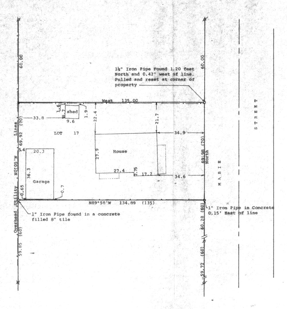
Scale = 1" = 20"ø= 1" Iron Pipe Found ⋈ = 3/4" Iron Pipe Found • = 2" Iron Pipe in Concrete found. top 2' above ground ------ Fence Line
