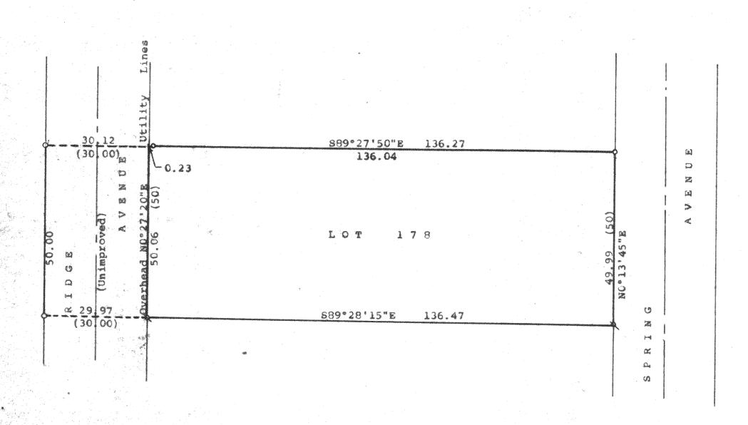
Scale - 1" = 20' N= 1" Iron Pipe Found o = 3/4" Iron Pipe Found (0.00) = recorded distance Bearings referenced to the assumed bearing of N0°27'20"E along the easterly line of Ridge Avenue. Survey ordered by: The Rauland Agency Walworth, WI 53184 Updating and recertification together with a survey of part of RidgenAvenue ordered by: Century 21, Skandia Realty 312 South 7th Street
