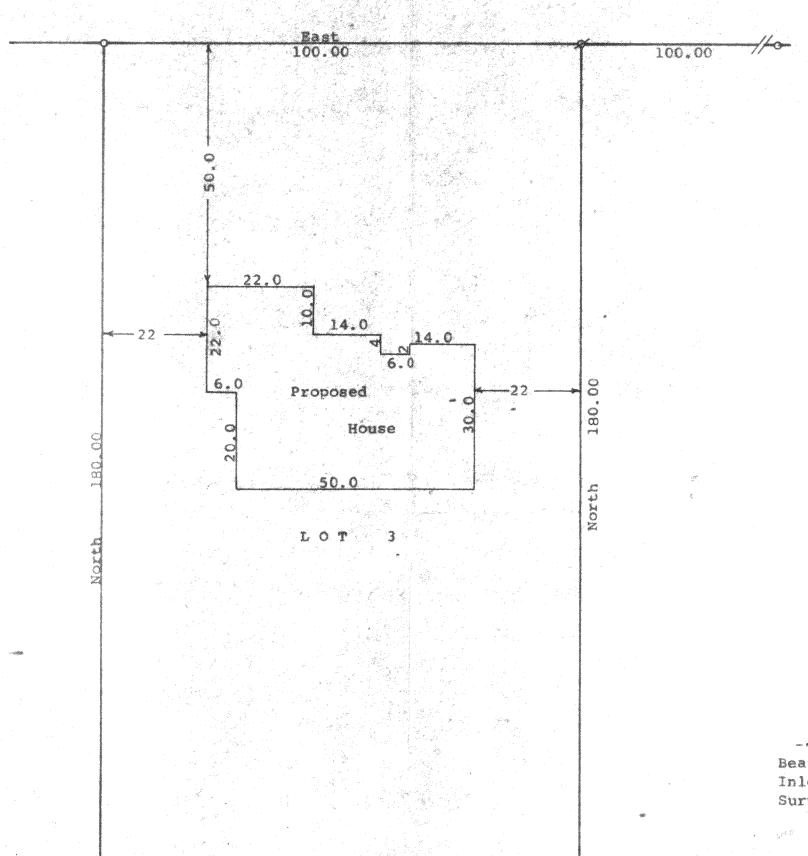
Scale - 1" = 20' 0 = 1" Iron Pipe Found Ø = bent 1" Iron Pipe Found. Pulled and reset 1" X 24" Iron Pipe ------ Qld Fence Line Bearings are those on the recorded plat of Inlet Oaks Subdivision No. 5 Survey ordered by: Gordon Nelson for Warren Bentley 7573 West Pleasant Delavan, WI 53115
