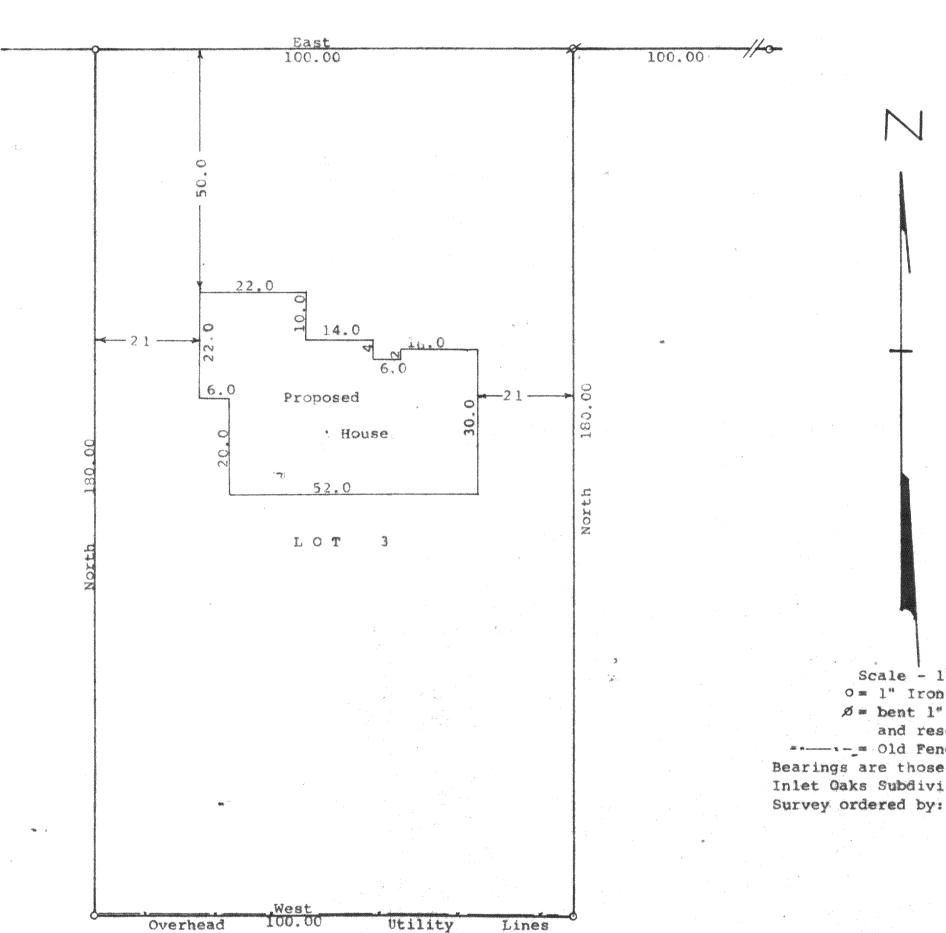
Scale - 1" = 20" O = 1" Iron Pipe Found Ø = bent l" Iron Pipe Found. Pulled and reset 1" X 24" Iron Pipe ------ Old Fence Line Bearings are those on the recorded plat of Inlet Caks Subdivision No. 5 Survey ordered by: Gordon Nelson for Warren Bentley 7573 West Pleasant Delavan, WI 53115
